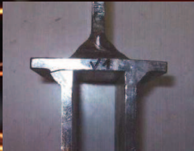
Figure 20: Physical test - crack along the weld leg
