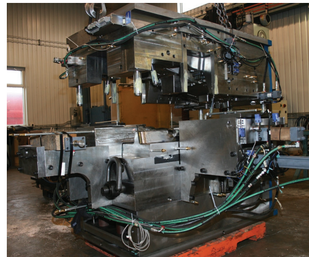
Completed mold assembly for BRP Piranha project – virtual and physical. Mold size: 62 x 37.5 x 42.5 inches; number of components: 900; press size: 1,600 tons.
