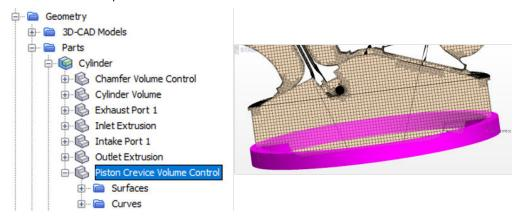
• STAR-ICE now automatically identifies the piston crevice region, and creates a volume control for mesh refinement that moves with the piston
